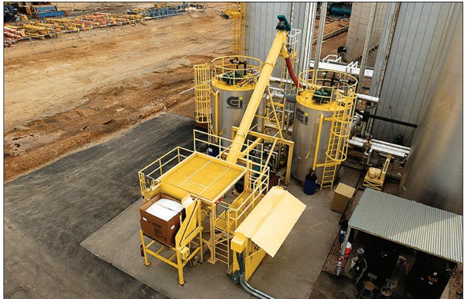
**Each batch of concentrate** requires about 3 to 4 hours for processing. Therefore, it is normal to have two parallel mixing tanks in the process to increase the system's production rate. The two-batch process also lends itself to higher quality control.
